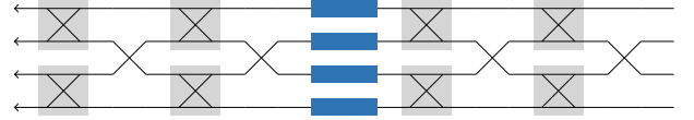
Figure 5: Datapath for a bit reversal on 2^n = 16 elements streamed on 2^k = 4 ports [17].
